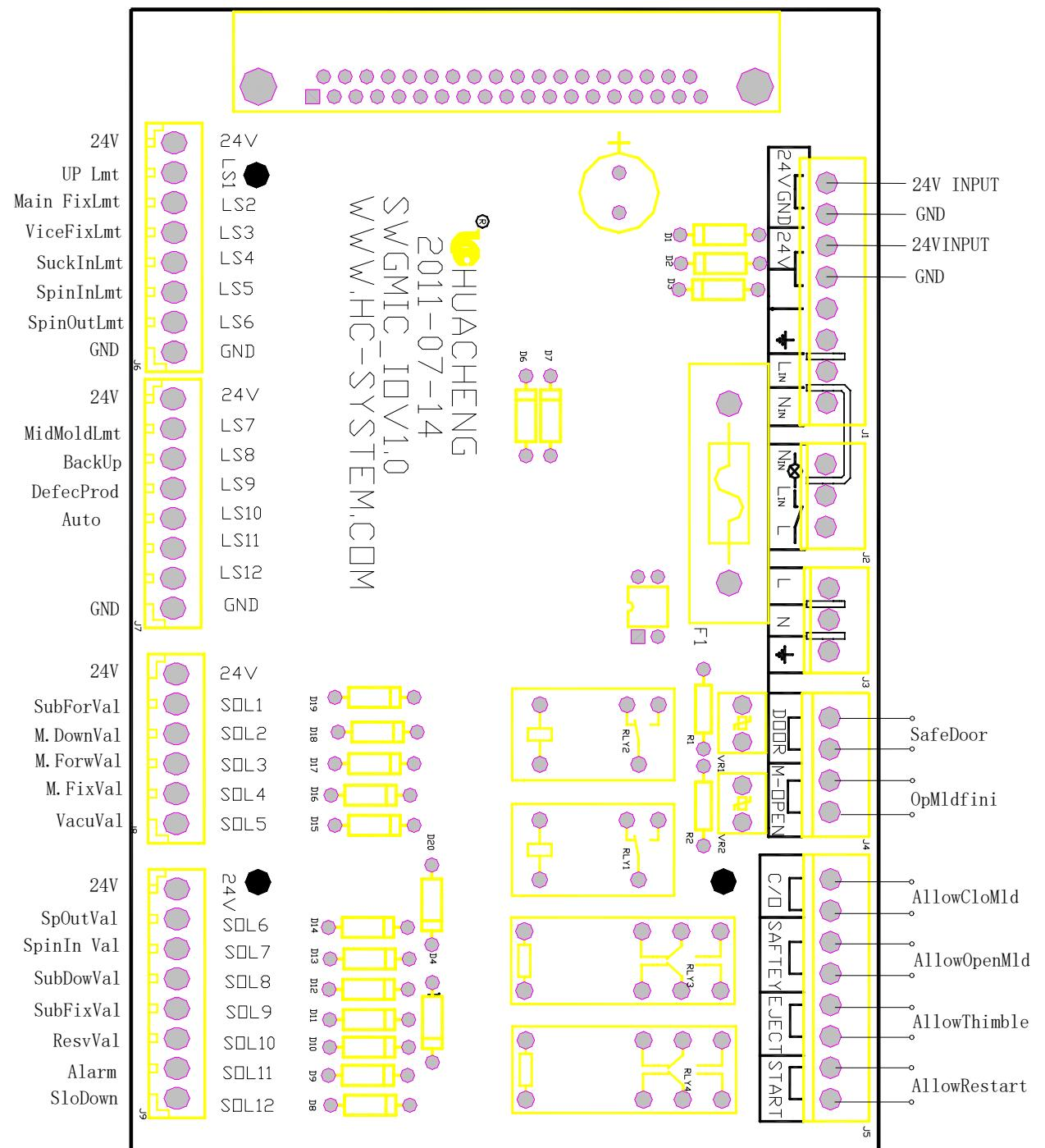
Conjunction with Injection machine diagrams
